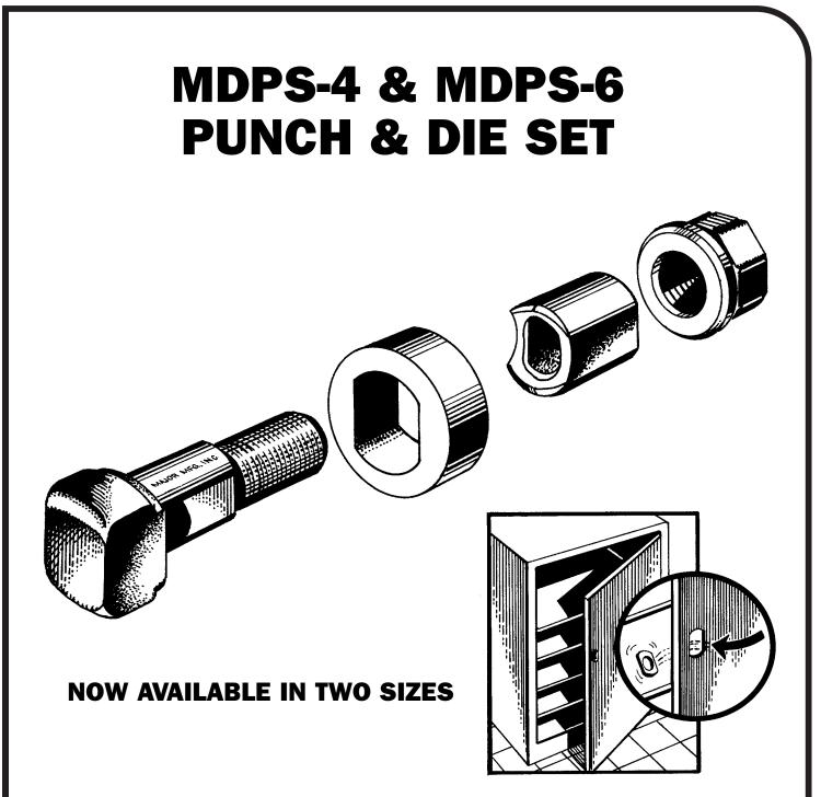
Major Manufacturing's punch and die set will punch a **DOUBLE "D"** hole in sheet metal cabinet drawers and doors. A must have tool for the locksmith working on vending machines, lockers, metal cabinets or any type of sheet metal door made with 18 guage (.048) or lighter steel. To use, simply drill a 1/2" hole centered where the cam lock is to be installed, slide the punch through the hole and tighten down the hex nut with a 11/16" wrench or socket set.
