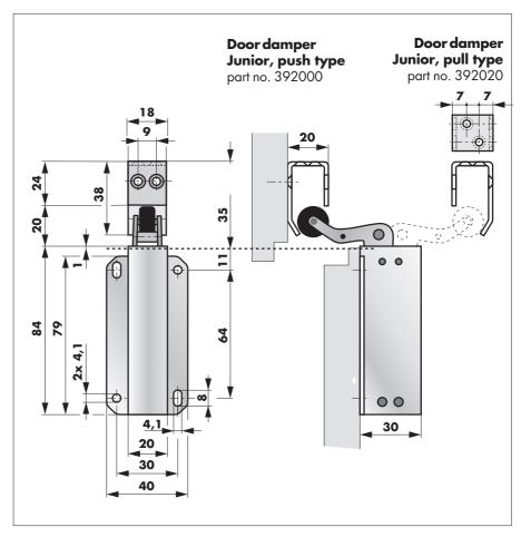
The door damper Junior pull type and push type just differ in the position of the operating lever with the rubber roller. The pull type has the operating lever fixed in the posterior holes of the casing and shows backwards (see dotted drawing). This type is used e.g. when the door damper is fixed to the back part of a drawer and the hook is fixed to the inner panel of the cupboard.
