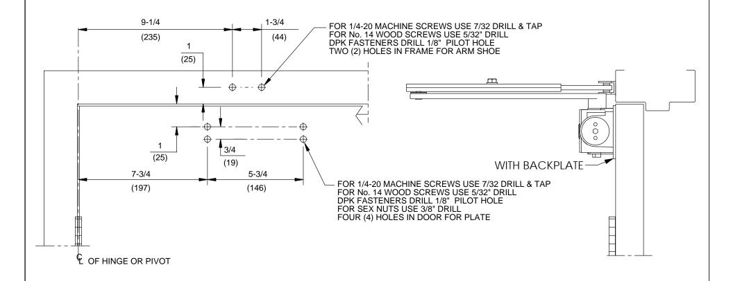
DOOR CLOSER MODELS: 8916, 8956 AF89, PH REGULAR INSTALLATION (PULL SIDE MOUNT) WITH PLATE BP89
