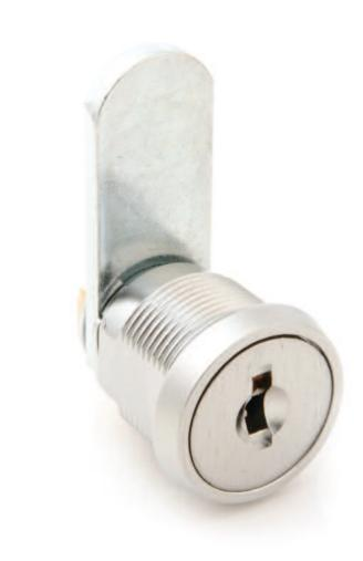
CCL Security Products offers multi-application single bitted Disc Tumbler Camlocks. These are diecast and can be Masterkeyed. All the locks are individually polybagged including a C2L straight cam and a C4L/C6L offset cam, the pronged washer, a 180 degree cam stop, and a collar ring.
