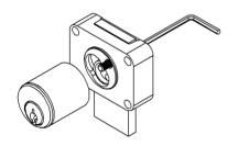
USE A 5/64 ALLEN WRENCH FROM THE BACK TO REMOVE THE CYLINDER.
