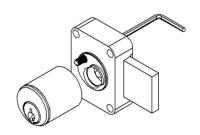
USE A 5/64 ALLEN WRENCH FROM THE BACK TO REMOVE THE CYLINDER.
