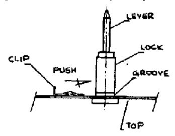
III) Hold lock in place and slide retaining clip behind top flange and push or hammer into grooves in lock.
