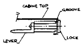
Install lock in hole with lever down. Lock lever must turn counter clockwise to lock cabinet. Lock lever must go through two fingers (tabs) on lock bar.
