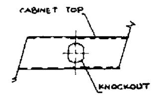
Remove knockout in top front flange using screwdriver and hammer.
